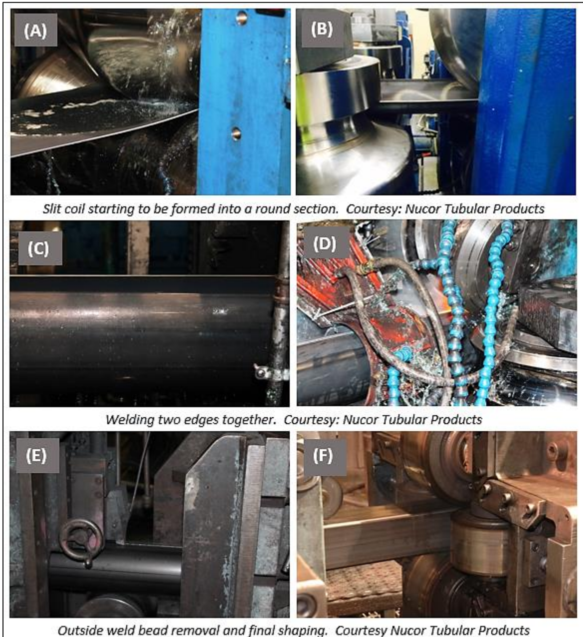
Figure 12: Continuous Forming HSS Shapes
