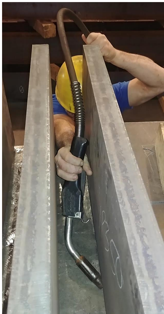
Figure 38: Welder Attempting Access to Plates with Poor Clearance
