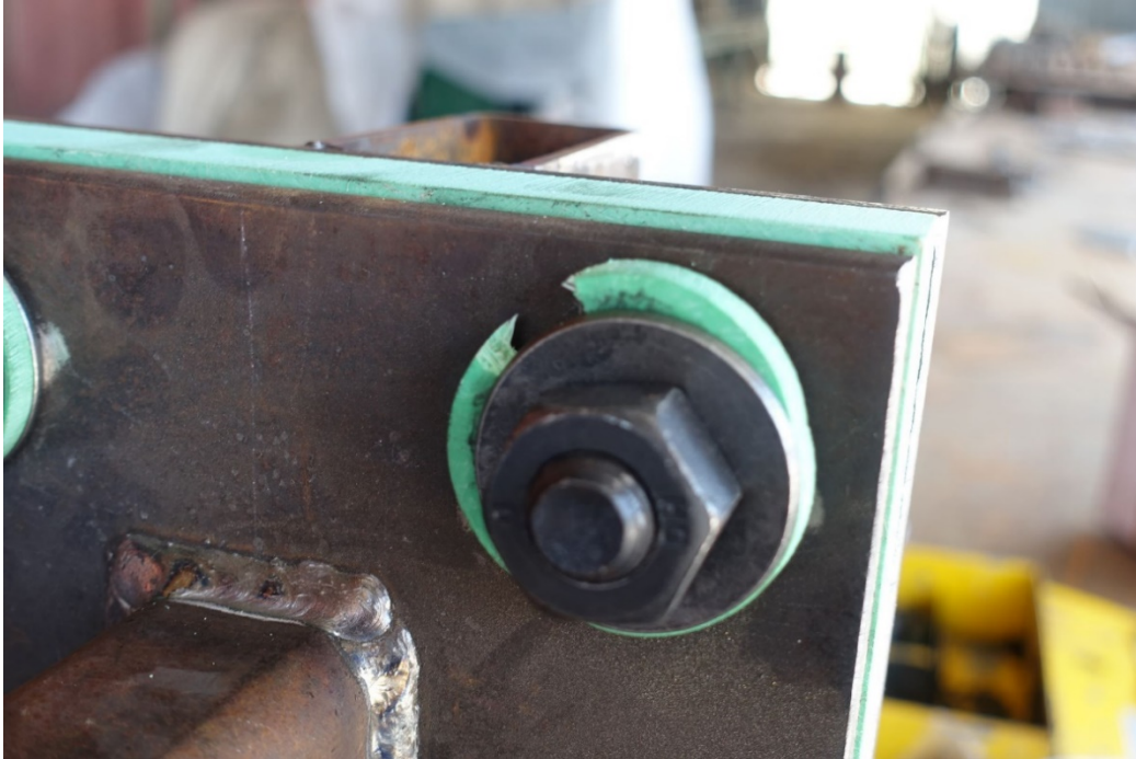
Photo 2: Thermal washer failure at Bolt #1 with regular oversized washer
