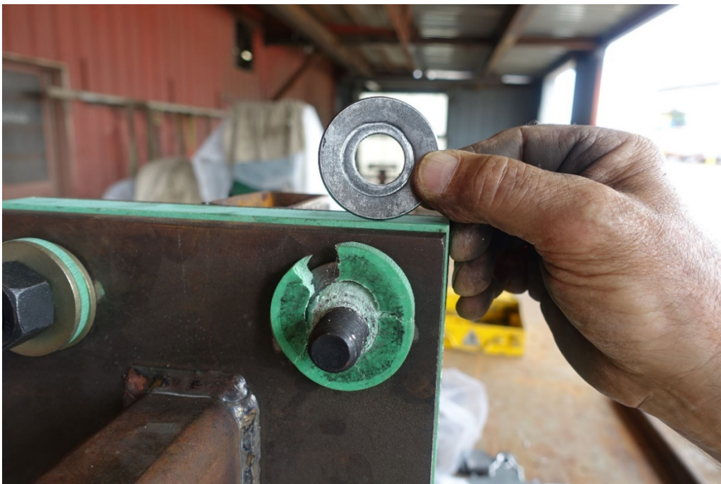
Photo 3: Thermal washer failure at Bolt #1 with regular oversized washer
